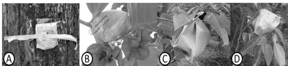
Figure 2. Images of the methods used to collect ^{137}\text{Cs} in stemflow and raindrop using a sphagnum pad. To collect the ^{137}\text{Cs} in stemflow, sphagnum pads were attached onto the trunk (A) of UWT and WT in the Japanese persimmon orchard and of UWT in the yuzu orchard. To collect the deposited ^{137}\text{Cs} , sphagnum pads were attached onto the calyx (B). To study the effect of deposited ^{137}\text{Cs} on the calyx and the concentration of ^{137}\text{Cs} in mature fruit, a fruit on a lateral branch was selected and a sphagnum pad attached and bagged, control (C) treatment. To collect the intercepted ^{137}\text{Cs} by leaves, sphagnum pads were attached onto leaves of the persimmon and the yuzu trees (D).
