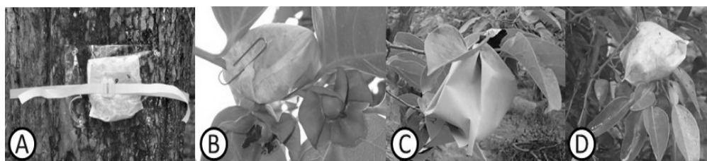
Figure 2. Images of the methods used to collect ^{137}\text{Cs} in stemflow and raindrop using a sphagnum pad. To collect the ^{137}\text{Cs} in stemflow, sphagnum pads were attached onto the trunk (A) of UWT and WT in the Japanese persimmon orchard and of UWT in the yuzu orchard. To collect the deposited ^{137}\text{Cs} , sphagnum pads were attached onto the calyx (B). To study the effect of deposited ^{137}\text{Cs} on the calyx and the concentration of ^{137}\text{Cs} in mature fruit, a fruit on a lateral branch was selected and a sphagnum pad attached and bagged, control treatment (C). To collect the intercepted ^{137}\text{Cs} by leaves, sphagnum pads were attached onto leaves of the persimmon and the yuzu trees (D).
