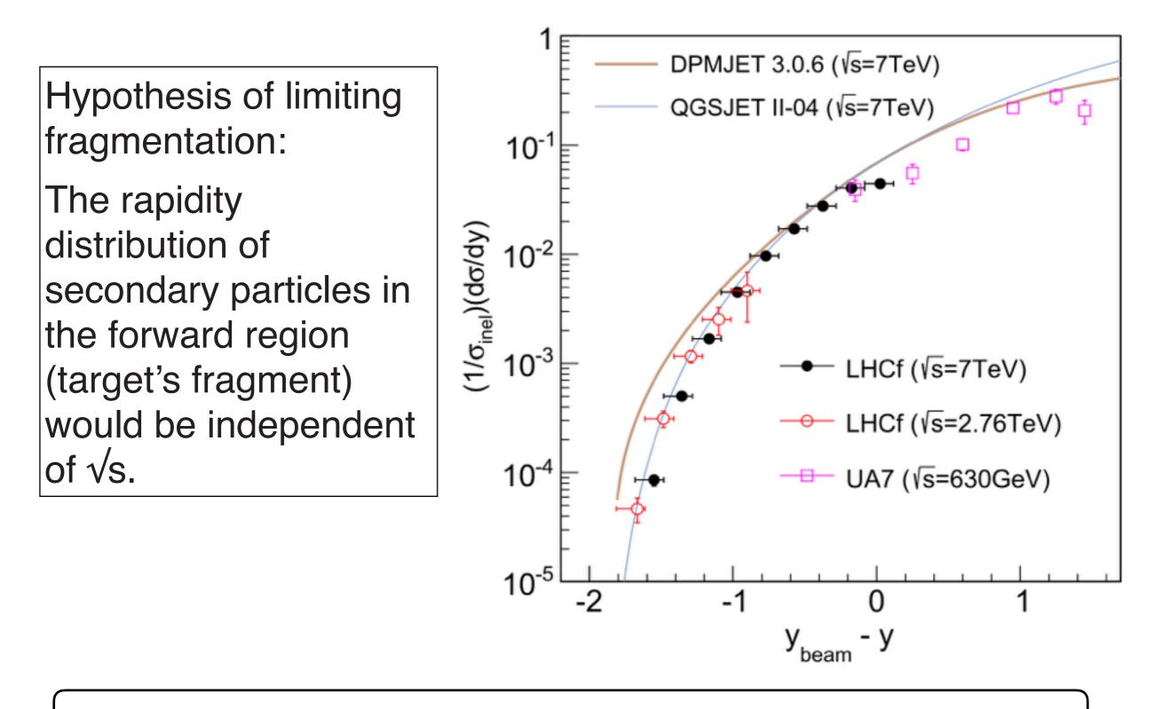
The scaling for forward  $\pi^0$  is true at the level of  $\pm 15\%$
