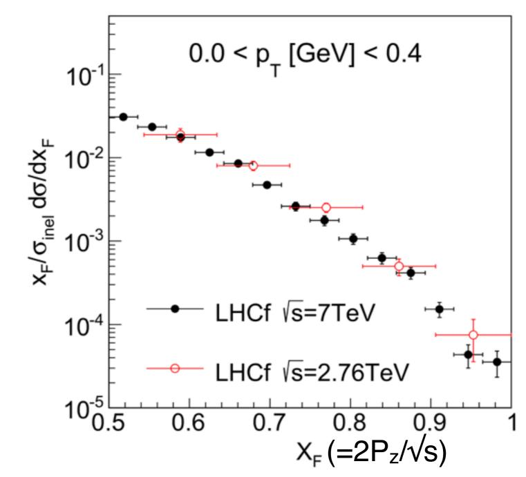
The Feynman scaling for forward  $\pi^0$  is true at the level of  $\pm 20\%$
