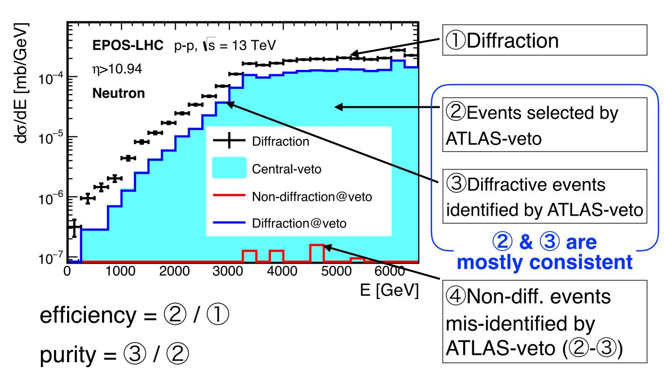
ATLAS-veto enable diffraction selection with high purity
