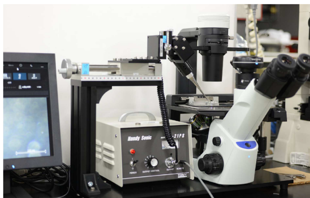
Fig. 2. New unroofing setup consisting of an inverted phase-contrast microscope equipped with a video camera, customized ultrasonic generator and an assistance device holding the horn-type probe in a hands-free manner.
