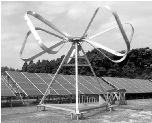
Fig. 5 Twist state of blades of Butterfly Wind Turbine observed in experiment driven by an induction motor
