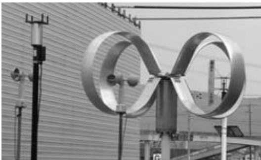
Fig. 9 Experimental rotor of the aluminum circular-blade butterfly wind turbine (ACBBWT)
