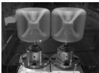
Fig. 4 Experimental setup of a pair of 3-D-printed VAWT models with a 5-mm gap (viewed from downstream)
