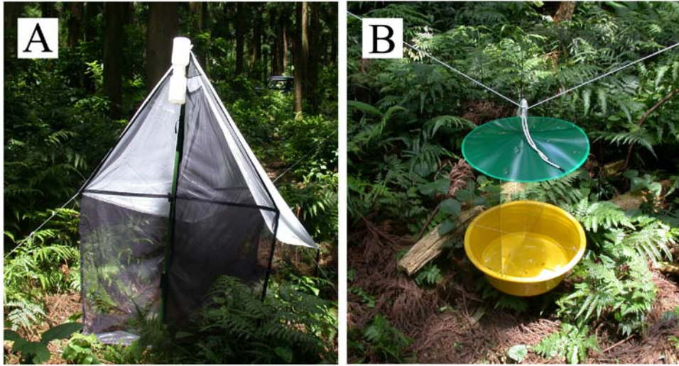
Figure 2. Collecting traps set in the site, plantation of Cryptomeria japonica in Kankake (CW). A: Townes-type Malaise traps. B: IBOY-type window trap.
