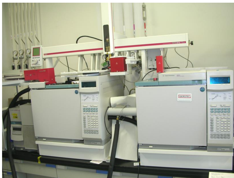
Figure 3-3. MD-GC-MS system using an Agilent 6890 gas chromatograph equipped with a first column, a multicolumn switching system, and an Agilent 6890 GC coupled to a MSD5973N quadrupole mass spectrometer equipped with a second column.
