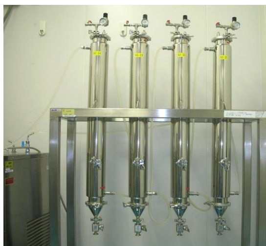
Figure 2-1. The 5-L stainless-steel tall tubes for fermentation, equipped with the strict controller of pressure and temperature.
