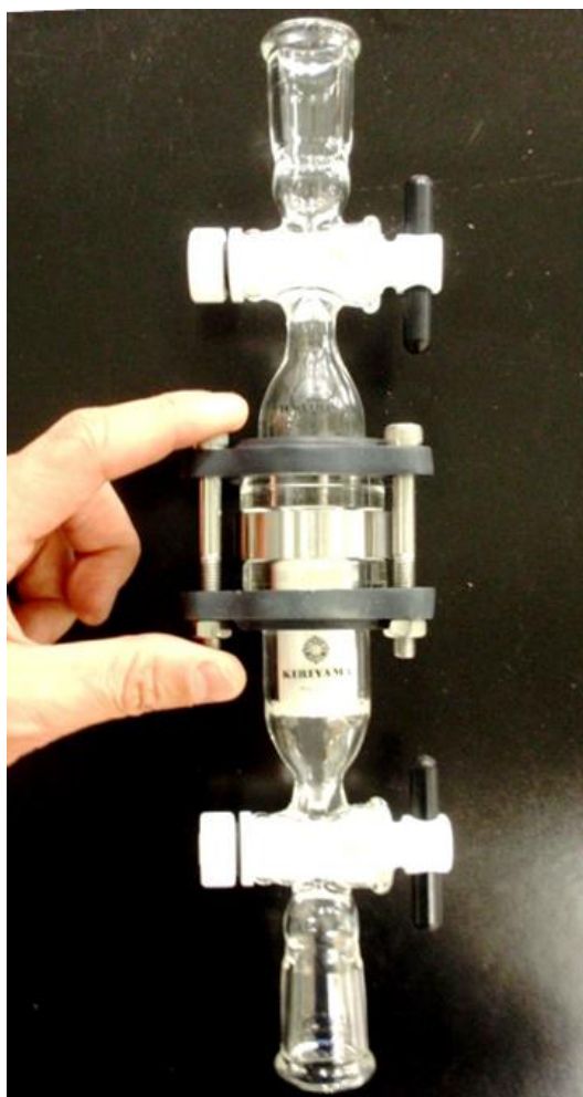
Figure 3-2. The elution column designed for the isolation of volatile thiols [101].
