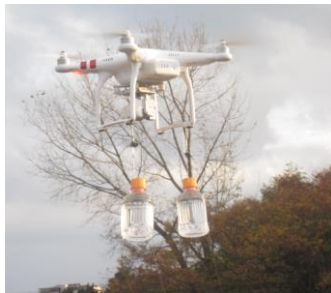
Fig.3 Experimental flight assessment with two bottles and fishing lines.
