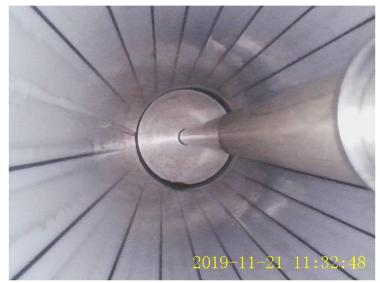
Fig.9. Endoscope photograph of the area near the electrodes taken inside the reactor after completion of the experiment.
