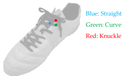
Figure 5. The mean coordinate value of impact point of each trial. Points of mean coordinate value of impact point are showed by color of blue, green and red respectively straight, curve and knuckle.
