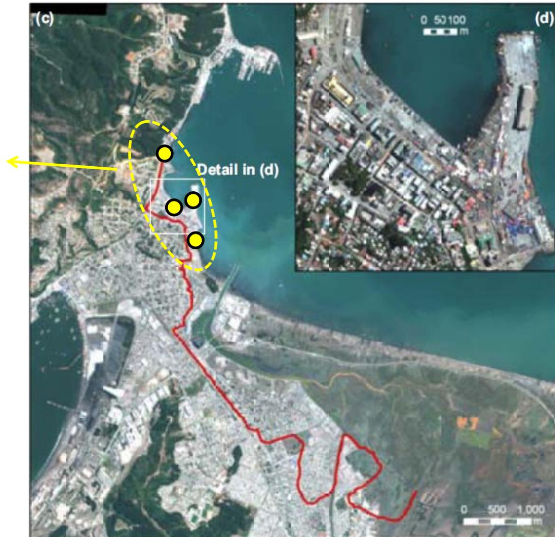
\*写真と浸水限界線(赤線)の出典: Koshimura S. and Matsuoka M.: Searching tsunami affected area by the 2010 Chilean earthquake tsunami by integration of tsunami numerical model and satellite images, Proceedings of the 8th International Workshop on Remote Sensing for Disaster Management, Tokyo, Sept. 30, 2010.
