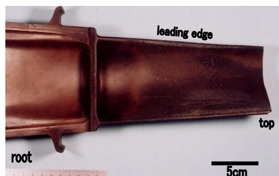
Fig. 1 First stage turbine blade
