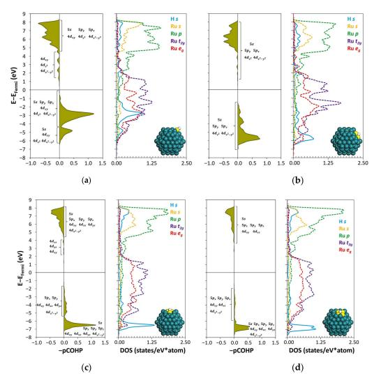
**Figure 3.** Bonding analyses of the H atom interacting on (**a**) top, (**b**) bridge, (**c**) 3F, and (**d**) 4F sites of Ru<sub>153</sub>. The projected crystal orbital Hamilton population and the density of states of the H atom (white sphere) interacting with the Ru atoms (yellow spheres) are shown.
