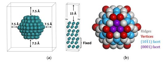
**Figure 4.** (**a**) Models of the Ru<sub>153</sub> nanoparticle and Ru(0001) and (**b**) distribution of Ru atoms at facets, ridges, and vertices.
