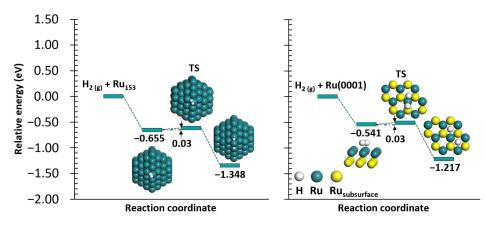
**Figure 2.**  $H_2$  dissociation on  $Ru_{153}$  and Ru(0001). Only the surface and subsurface Ru atoms are shown for the  $H_2$  dissociation on Ru(0001). The TS and energy barrier are also shown.
