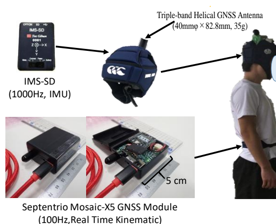
Fig. 1 Configuration of GNSS and IMU attachment on rugby headgear
