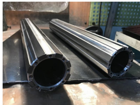
Fig. 2 HOPG bonded to the inner cylinder of the spindle shaft.
