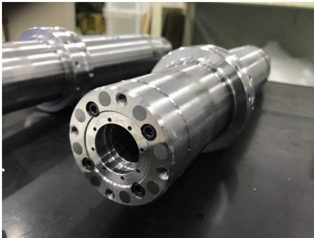
Fig. 4 Visual indication of a spindle shaft in which HOPG is bonded to carbon steel.
