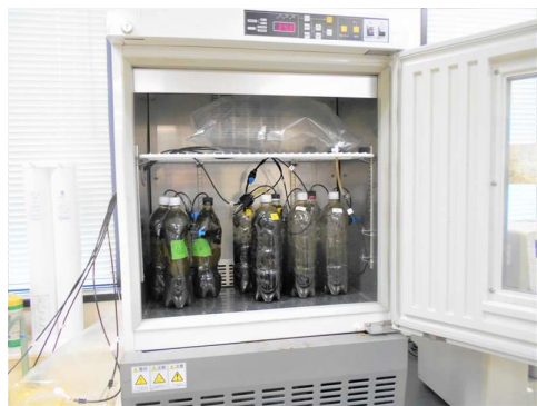
Fig.3 Methane production test from sweet potato and sewage sludge using PET bottles.
