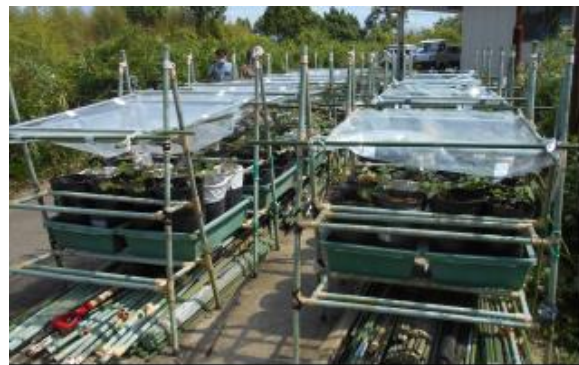
Fig. 3 Cultivation test method using UV/heat ray shielding sheets.
