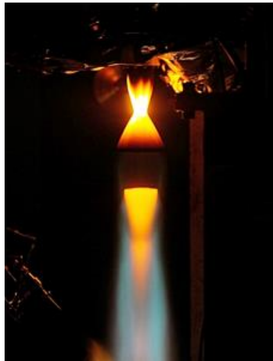
Figure 2 SiC/SiC combustion chamber and nozzle operating under vacuum.
