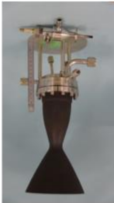
Figure 1 SiC/SiC combustion chamber and nozzle equipped with core engine.
