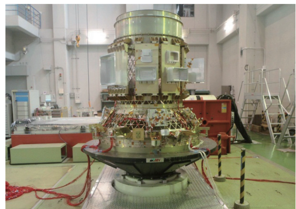
Fig. 9. Vibration test of the PBS that was conducted at ISAS/JAXA Sagamihara campus in 2012. Note, PAF is installed atop the PBS.
