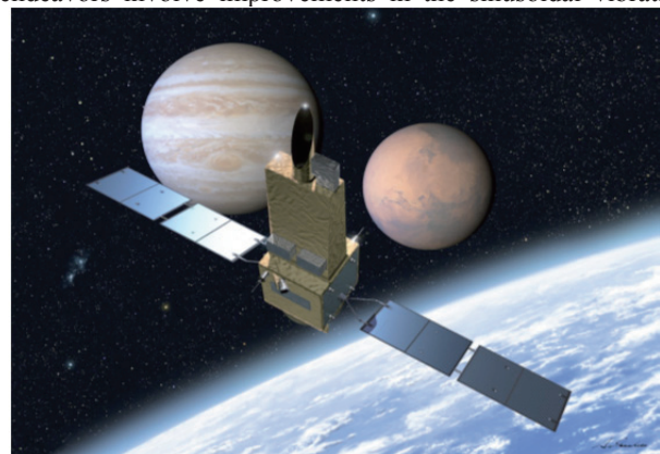
Fig. 1. Artistic view of SPRINT-A, an extreme ultraviolet planetary telescope to be onboard the first flight of Epsilon. It weighs 320 kg.
