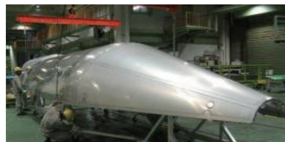
Fig. 5. Payload fairing of Epsilon in the final process of manufacturing.
