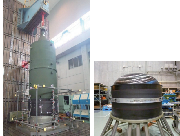
Fig. 4. Qualification Tests (QT) of the Epsilon's second stage motor: the mechanical test conducted at ISAS/JAXA Sagami campus (left) and the pressure test at Tomioka factory of IHI Aerospace Co. Ltd. (right) both executed in the first quarter of 2012.
