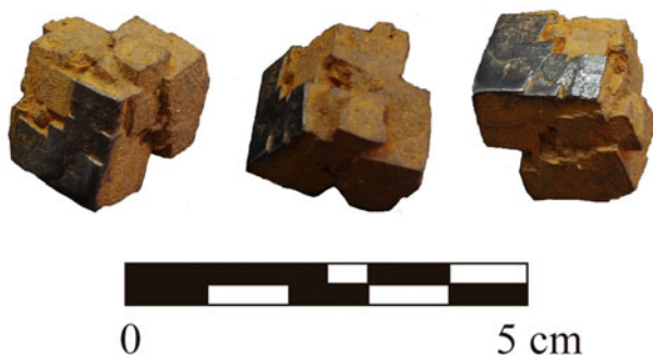
Figure 4. Raw material from Cancuen (sample CAN-2). Note the cubic crystal habit, and the luster and color exposed in the polished facet. Photos by Carías.
