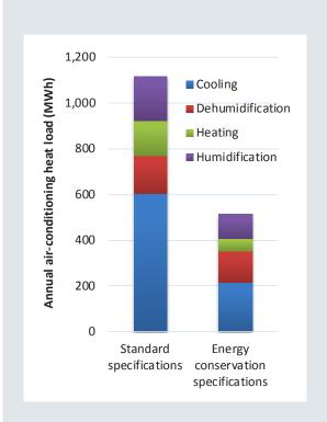
Figure 1. Comparison of annual integral heat load values of model buildings.
