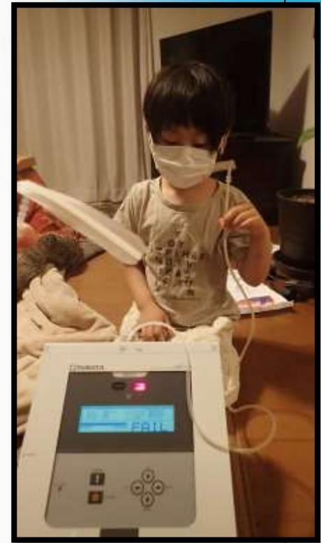
Fig.2 The appearance of fit test with the Mask Fitting Tester Model MT-03™, Roken type
