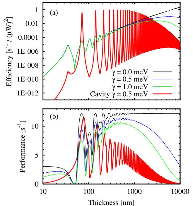
FIG. 3: Thickness dependence of (a) generation efficiency  $S/I^2$  and (b) performance  $P$ . Dielectric constant of outside is  $\epsilon_{\text{bg}}$ , scattering frequencies are the same as that of pumping field, and scattering is forward with  $\theta = 0^\circ$  (black, blue, and green). The red lines represent backward emission from a CuCl film with an optical cavity, whose mode frequency is tuned to  $\omega_T$ .
